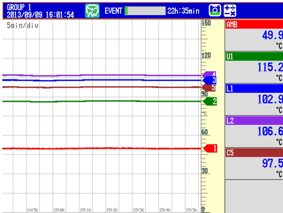
Figure 16 – Thermal Measurement at 132 VAC Input, ~50 °C Ambient.
